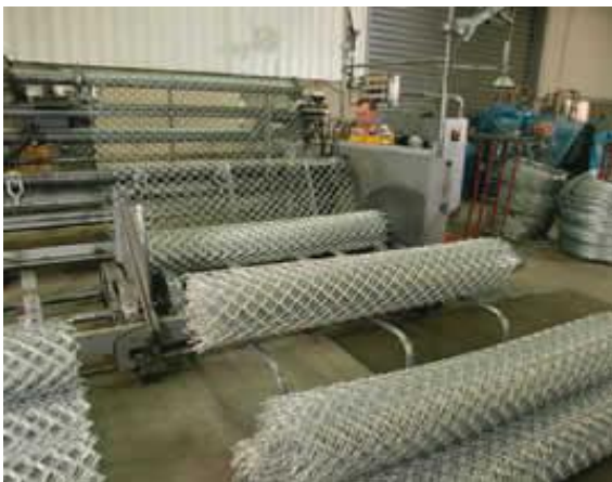
Chain link machine and chain link fence
