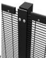
The Bekasecure post's design and high yield strength steel provide the ultimate in high security, rigidity and ease of installation. Posts are foreseen with a double range of wholes 10 x 20 mm and the fixation of the panels is secured by the use of a continuous cover plate and specific inox security bolts. The open profile of the post allows electrical or fibre optic cabling and is closed with specific metal cap.
